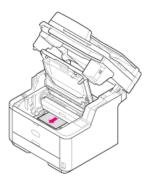
• If the bottom end of the paper is visible, pull out the paper in the direction of the arrow gently while holding its top end.
