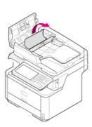
• If the top end of the document is visible under the paper guide, lift the paper guide.
