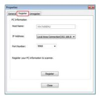
After installing the scanner driver, start Network Configuration, and then select a driver to use. Select [Properties] from the [Scanner] menu, and then select the [Register] tab. As the computer information, the computer name, IP address and port number are displayed. You do not need to set the computer name, because the computer's host name is automatically acquired.
