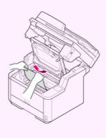
• If the bottom end of the paper is not visible but its top end is visible in the paper output unit, pull out the paper gently while holding its top end.
