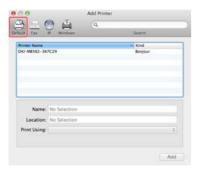
10. Select the machine with [Kind] being [Bonjour], and then check that [OKI MB562(PS)] is displayed for [Printer Name].
