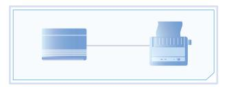
Station Message Detail Recording (SMDR) automatically prints out detailed call information for outside calls. A printer connected to the Serial Interface (RS-232C) port can be used to print incoming and outgoing outside calls, as well as print a hard copy of system programming.
