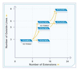
Panasonic offers you unprecedented flexibility and simple expansion with optional cards. By adding optional cards, you can expand the system up to 8 COs / 24\* extensions to meet your changing needs. No additional programming and costly rewiring are required.
