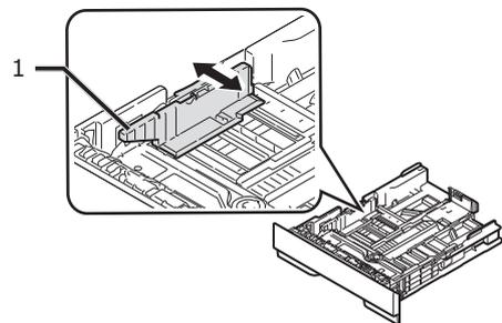
3 Slide the paper stopper (2) to the length of the paper to be loaded.
