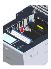
Turn the lock levers (c) on the both sides of the belt unit backward.
