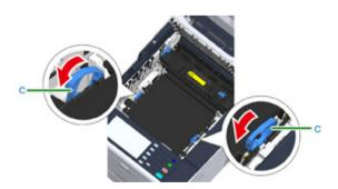
7 Remove the belt unit by holding the lock lever (c).
