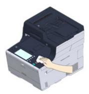
3 Dry the surface of the machine with a dry soft cloth.
