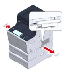
5 Lift up the machine to remove the additional tray unit.
