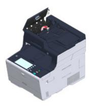
Wipe the document feeding rollers with a soft cloth lightly moistened with water. Wipe the whole surface of the roller while turning it with your hand.
