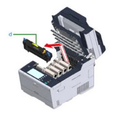
Hold the handle of a new fuser unit, align the fuser unit to the grooves behind the toner cartridges, place the fuser unit into the machine.
