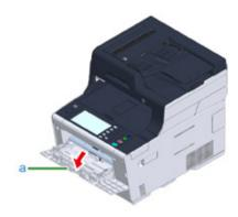
2 Slightly lifting the MP tray (a), press the right arm (b) inward, then unlock the tab (c).
