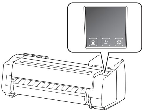
Guidance on how to change the ink, paper, and the print head appears on the operation panel touch screen. Replace the respective items by following the directions given by the guidance.
