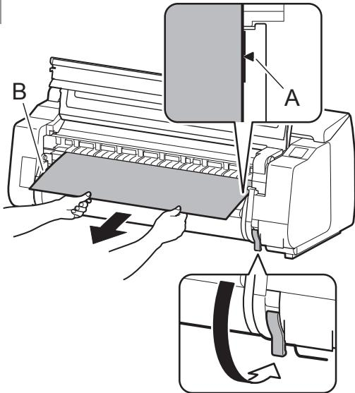
① Pull the roll paper out to the position of the output guide (B) so that the right edge of the roll paper is parallel to the line (A) and lower the release lever.
