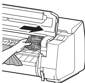
② If the carriage is out, manually move the carriage out of the way, away from the paper.
