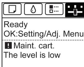
If a message is displayed requesting Maintenance Cartridge replacement, you can skip the step **Access the menu for Maintenance Cartridge replacement**. Follow the instructions in **Replace the Maintenance Cartridge**.
