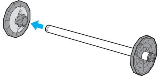
**2** Insert the attachments for the roll paper on the Roll Holder.
