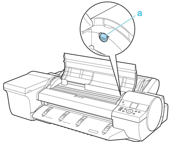
**4** Using the back of the Cleaning Brush, move the first Switch to the side opposite ●.
