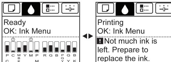
If a message requests you to replace an Ink Tank, press the **OK** button. In this case, you can skip the step **Access the menu for ink tank replacement**. Follow the instructions in **Remove the ink tanks**.
