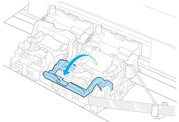
**4** Pull up the Printhead Fixer Cover to open it completely.
