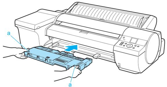
**8** Hold the Ejection Guide on both sides by the near end. Aligning the Ejection Guide with the guides (a), insert it into the printer until it locks in place.
