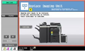
If a Toner Cartridge other than for black or the Imaging Unit is empty, printing can continue using black. Press [Continue], and then select the job to be printed.
