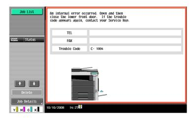
If a defective part can be separated in order to be able to continue operations after a problem has been detected, [Continue] or [Recover Data] is displayed. To continue operations, select any key. However, the problem has not been resolved, so contact your service representative immediately.
