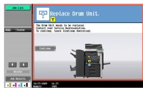
If a **Toner Cartridge** other than for black or the **Drum Unit** is empty, printing can continue using black. Press [Continue], and then select the job to be printed.
