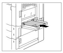
3 Slide the **Lateral Guide** to fit the size of paper being loaded.
