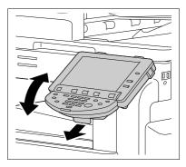
To tilt the **Control Panel** to the left or right, hold the bottom of the **Control Panel**, and then tilt the panel to the left or right.
