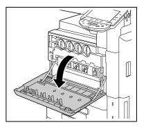
Release the Waste Toner Box Lock Lever, and then remove the Waste Toner Box.
