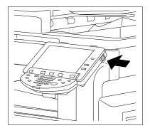
4 To turn the power off, press the **Sub Power Switch**, then the **Main Power Switch**.
