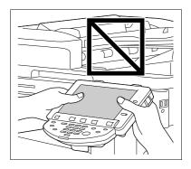
Pull the **Control Panel Release Lever** toward you, and then pull the **Control Panel** up or down.
