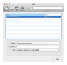
The printer driver for the selected printer is displayed in [Print Using:].
