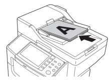
→ Load the original by positioning its top side to the left. When loading in a different orientation, be sure to specify the loading direction of originals.
