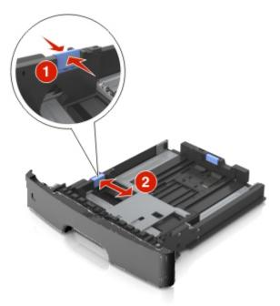
3. Unlock the length guide. Squeeze, and then slide the length guide tab to the correct position for the size of the paper you are loading.
