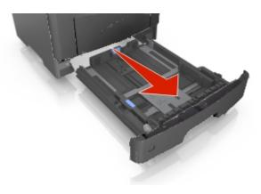
2. Squeeze, and then slide the width guide tab to the correct position for the size of the paper you are loading.
