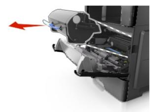
3. Lift the blue handle, and then pull the imaging unit out of the printer.
