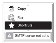
• If [Fax] has been enabled in step 4 of the setup procedure, a warning message is displayed on the **Control Panel** screen to notify you that the fax line is not connected. This message is not displayed if a modular cable is connected to this machine.
