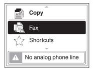
If you are not going to use the fax function that has been set to be enabled, select [Settings] - [Settings] - [Fax Settings] - [Analog Fax Setup] - [General Fax Settings] - [Enable Line Connected Detection] - [Off] on this machine, and press the **OK** button.
