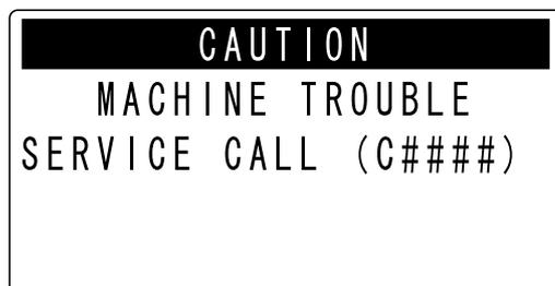
If this message appears in the **Display**, turn off the power switch, wait for about 10 seconds, then turn on the power switch again.
