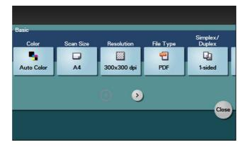
→ Before scanning the original on this machine, specify the size of the original to be scanned. If you fail to set the original size correctly, the image may be cut off. For details on how to specify the original size, refer to page 1-12.
