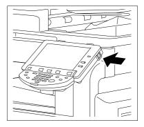
To turn the power off, press the **Sub Power Switch**, then the **Main Power Switch**.
