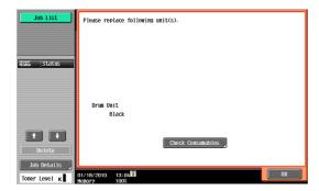
If a user continues to operate the machine while a warning message is displayed, the following replacement message appears. Replace the **Toner Bottle** according to the guidance contained in your maintenance agreement. For **Drum Unit**, contact your service representative.
