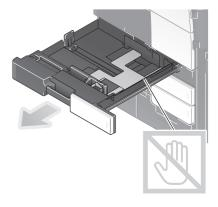
Slide the Lateral Guide to fit the size of the paper to be loaded
