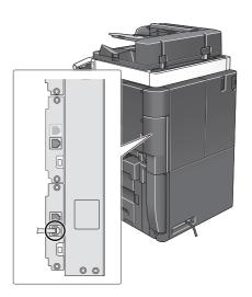
Check that a LAN cable is connected to the LAN port of this machine and the green LED is on.
