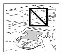
1 Pull the Control Panel Release Lever toward you, and then pull the Control Panel up or down.
