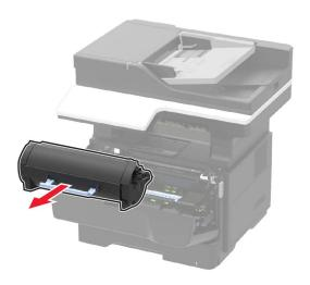
**3** Remove the used imaging unit.
