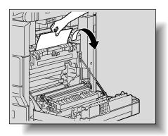
Decreased copy quality may result if the surface of the image transfer roller is touched. Be careful not to touch the surface of the image transfer roller.
