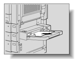
If misfed paper cannot be pulled out, pull the lever for the sliding plate of the bypass tray, and then pull the sliding plate toward you.
