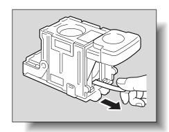
7 Insert the staple cartridge holder, and then push it down until it locks into place.
