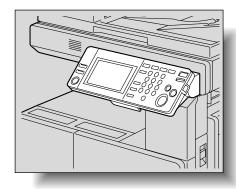
To return the control panel to the upper position, pull the control panel release lever toward you, and then pull up on the control panel.
