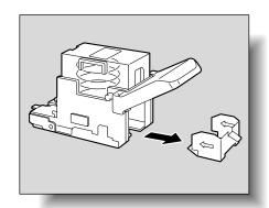
4 Load the new staple cartridge into the staple cartridge holder.
