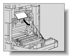
6 Carefully pull out any misfed paper in the fusing section.
