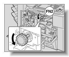
4 If the punch unit is installed, pull out the hole-punch waste container.
