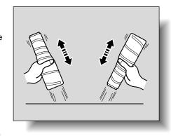
toner is mostly broken up before installing the bottle.
