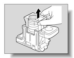
4 Remove the empty staple cartridge from the staple cartridge holder.
