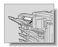
4 Open the misfeedclearing door, and then pull out any misfed paper.
