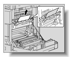
Open the switching guide, and then carefully pull out any misfed paper in the switchback unit.
