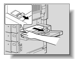
3 Press down on the sliding plate with your left hand and carefully pull out any misfed paper.
