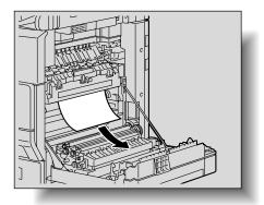
7 Carefully pull out any misfed paper around the image transfer roller.
