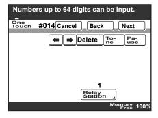
9 To change the relay machine, touch [Relay Station], and then select the desired relay station.
