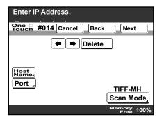
9 To select the file format and coding method, touch [Scan Mode].
