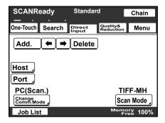
7 To select the file format and coding method, touch [Scan Mode].
