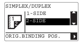
→ When you select [2-SIDE] and press the ► key, you can specify the binding direction of the original. Select [LEFT] or [TOP], then press the OK key.
