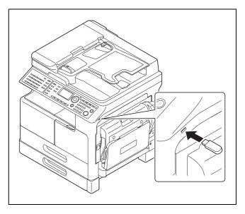
3 Use the ▲/▼ key to select [SCAN TO USB], then press the **OK** key.
