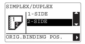
→ When you select [2-SIDE] and press the ▶ key, you can specify the binding direction of the original. Select [LEFT] or [TOP], then press the **OK** key.
