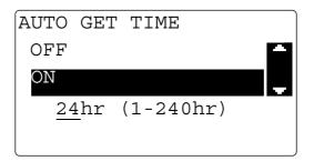
Enter time using the **keypad**, then press the **OK** key.
