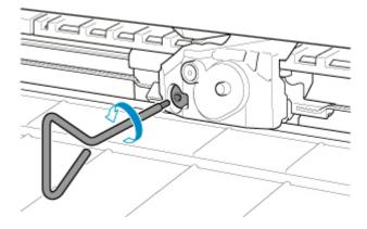
6. Remove cutter blade while holding A.
