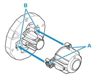
5. Insert holder stopper from left into roll holder as shown, and then while holding in position (B), push firmly until holder stopper flange (A) touches roll paper. Lock the holder stopper lever (C) by rotating it towards .
