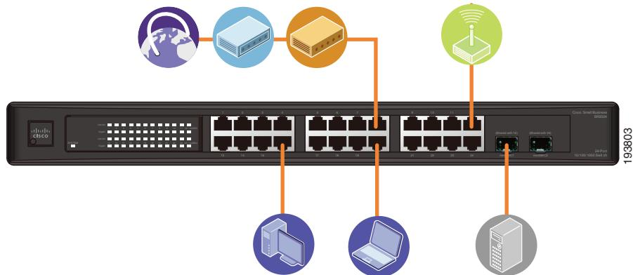
**To connect network devices** (such as gateways or other switches) to your unmanaged desktop switch you need one suitable Twisted Pair (TP) cable for each unit. We recommend Category 5 or better cable for Gigabit connections.
