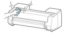
• Open top cover and output guide and clean parts that come in contact with paper (A, B).
