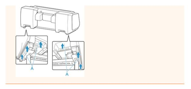
2. Remove tape and packaging material attached to the printer. Also open the top cover and remove stoppers and spacers inside the printer.
