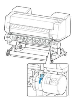
7. Hold flanges (A) so that roll holder's white gear is on left, align roll holder shaft with roll holder slot left and right guide grooves (B), and load.
