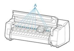
4. While pressing button (A) in center of print head lock lever, pull it forward to open it until it stops.
