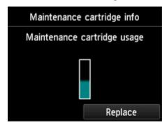
If the touch screen indicates to replace the maintenance cartridge, replace the maintenance cartridge. If a message appears indicating to check the remaining capacity of the maintenance cartridge, or before tasks that deplete much of the capacity such as head cleaning or preparations to move the printer, check the remaining maintenance cartridge capacity and prepare a new maintenance cartridge as needed.
