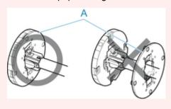
2. If using 3-inch core paper, align 3-Inch Paper Core Attachment tabs (A) with Roll Holder holes (B) and insert firmly.
