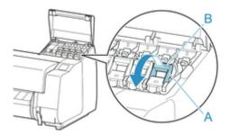
3. Lift ink tank lock lever until it stops, and then push it down toward front.
