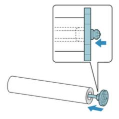
3. Load roll paper in printer or roll unit. (See "Loading the Upper Roll on the Printer.") (See "Loading the Lower Roll on the Roll Unit (Option).")
