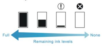
If the touch screen indicates to replace the ink tank, replace the ink tank. If a message is displayed indicating to check the remaining ink levels, or after tasks that consume a lot of ink such as large-format printing or head cleaning, check the remaining levels and replace ink tank as needed.
