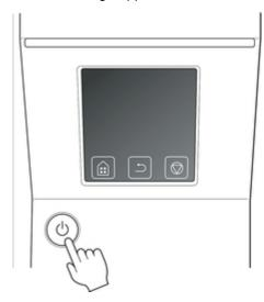
2. When startup is finished, **ON** button lights up, and printer enters standby mode.
