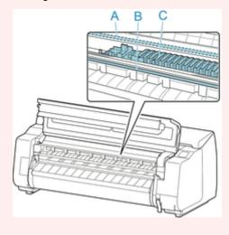
3. If ventilation duct (A) is dirty, use damp cloth that you have wrung out completely to wipe it clean.
