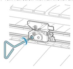
4. Remove cutter blade while holding A.
