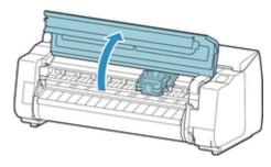
2. If the print head locking cover and print head lock lever are dirty, use a damp cloth that you have wrung out completely to wipe them clean.
