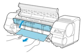
After removing the paper, inspect the interior to ensure paper fragments or other objects do not remain, and lower the output guide.
