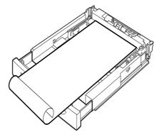
**3.** Push the paper tray completely into the printer.
