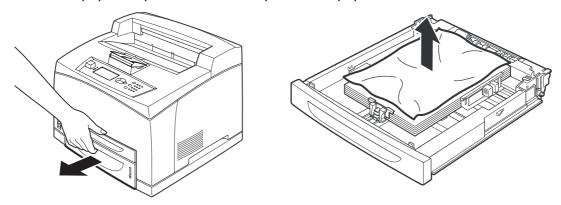
**2.** Examine the inside of the printer and remove any jammed paper.
