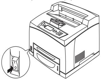
2. When the power is switched on, various screens will be displayed on the control panel. Check that this display changes to Ready To Print.
