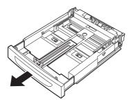
**5.** Squeeze the length guide and slide it to the desired paper size (1). Squeeze the right width guide and slide it to the desired paper size (2).
