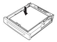
**7.** Close the lid of the paper tray and push the tray completely into the printer.
