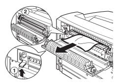
**3.** Raise the lever as shown in the diagram and open the cover B (1).
