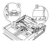
**6.** Load the paper with the side to be printed facing up and with all four corners aligned.
