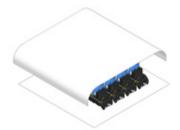
7 Open the transparent cover (c) inside the machine, remove the jammed paper slowly by pulling the edge of paper.
