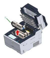
Hold the cartridge, pinch the tip of blue lever (d) of the toner cartridge, and turn it toward you until the tip aligns on the lug of the cartridge.
