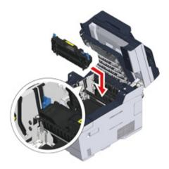
15 Tilt the lock levers (c) on the both sides of the fuser unit.
