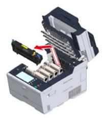
**9** Push the blue lever on the fuser unit and remove the safety stopper.
