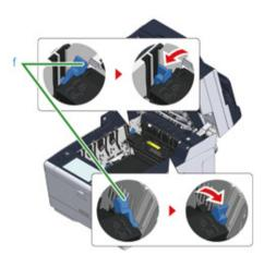
Hold the fuser unit handle and lift the fuser unit out of the machine.
