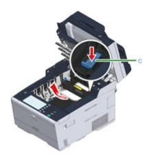
? Tilt back the lock levers (d) on the both sides of the fuser unit toward you.
