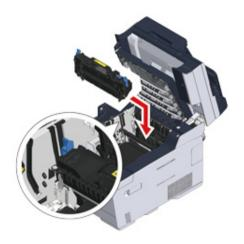
Tilt the lock levers (f) on the both sides of the fuser unit.
