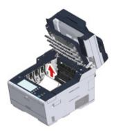
19 Hold the lock levers of belt unit and place the belt unit into the machine.
