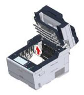
12 Hold the lock levers of belt unit and place the belt unit into the machine.
