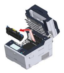
Turn the lock levers (g) on the both sides of the belt unit toward you and remove the belt unit by holding the lock levers.
