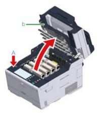
A Remove the four image drums from the machine and place the image drums on a flat surface.
