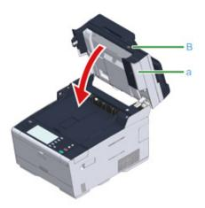
Do not close the scanner unit vigorously. It may cause the document feed roller of ADF to fall and get in the way of loading documents.
