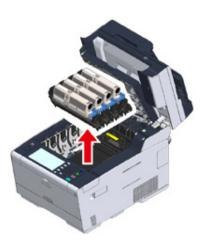
Cover the removed image drums with paper so that the image drums are not exposed to light.
