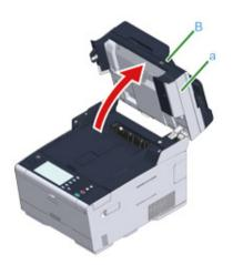
Press the button (A) and open the output tray (b) completely.
