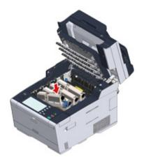
Hold the cartridge, pinch the tip of blue lever (c) of the toner cartridge, and turn forward until the tip aligns on the lug of the cartridge.
