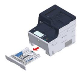
Slide the paper guide (a) to the width of paper to be loaded.
