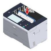
Turn the lock levers (e) on the both sides of the belt unit forward.
