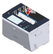
13 Turn the lock levers (g) on the both sides of the belt unit forward.
