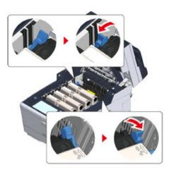
Hold the fuser unit handle and lift the fuser unit out of the machine.
