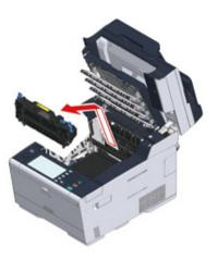
Turn the lock levers (e) on the both sides of the belt unit toward you and remove the belt unit by holding the lock levers.
