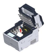
If paper jams in the fuser unit, press the jam release lever (e) on the fuser unit and slowly pull the jammed paper toward you.
