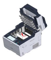
Hold the fuser unit handle and place the fuser unit into the machine.
