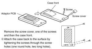
③ After connecting the cables (refer to the following sections), replace the case front. Be careful not to damage the wiring in the case.
