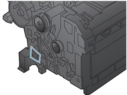
3. Examine the surface of the imaging drum on the bottom of the toner cartridge.
