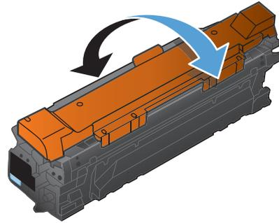
5. Remove the plastic shield from the toner cartridge.
