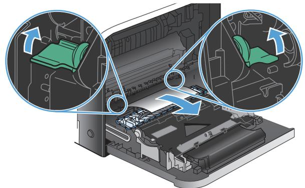
8. If paper is visible entering the bottom of the fuser, gently pull downward to remove it.
