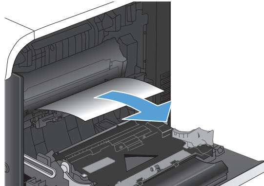
7. Look for paper in the Tray 2 roller area. Push up on the two green tabs to release the jam-access door. Remove any jammed paper, and close the door.
