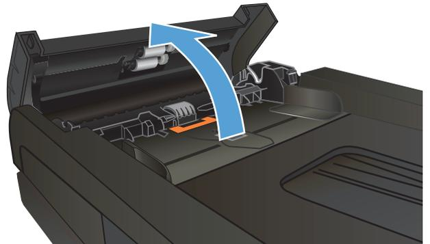
2. Use a moist, lint-free cloth to wipe both pickup rollers and the separation pad to remove dirt.
