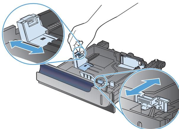
3. Load paper into the tray face-up. Check the paper to verify the guides lightly touch the stack, but do not bend it.
