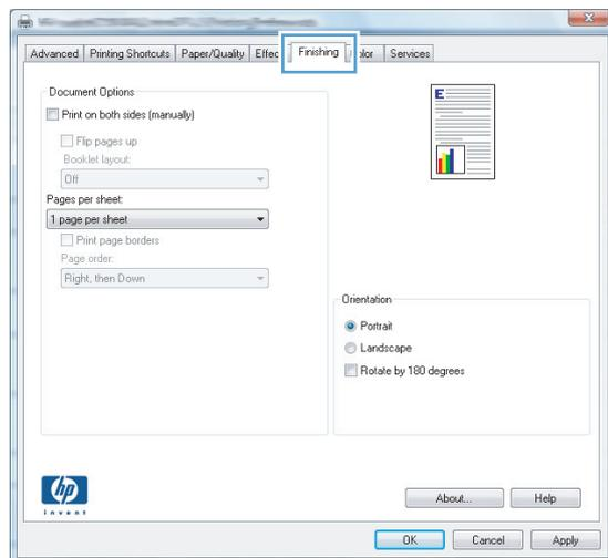
4. Select the **Print on both sides (manually)** check box. Click the **OK** button to print the first side of the job.
