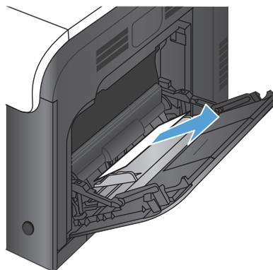
2. If you cannot remove the paper, or if no jammed paper is visible in Tray 1, close Tray 1 and open the right door.
