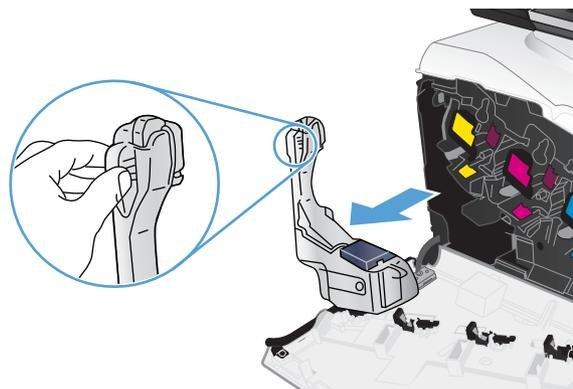
3. Place the attached blue cap over the blue opening at the top of the unit.
