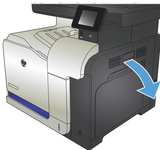
3. If paper is visible inside the right door, gently pull the trailing edge to remove it.
