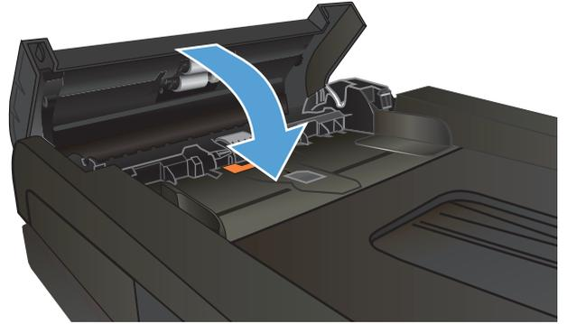
4. Open the scanner lid. If paper is jammed in the scanner lid, gently pull it out.
