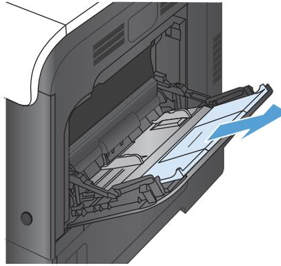
3. Fold out the tray extension to support the paper and open the side guides.
