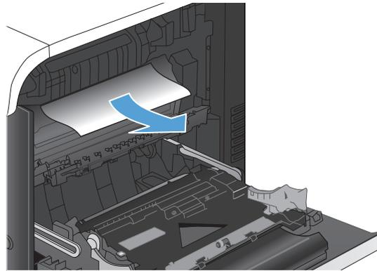
9. Paper could be jammed inside the fuser where it would not be visible. Grasp the fuser handles, lift up slightly, and pull straight out to remove the fuser.
