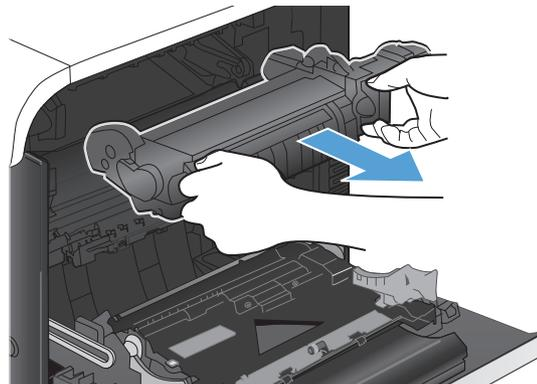
10. Open the jam-access door (callout 1). If paper is jammed inside the fuser, gently pull it straight up to remove it (callout 2). If the paper tears, remove all paper fragments.
