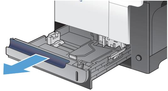
2. Adjust the paper-length and paper-width guides by squeezing the adjustment latch and sliding the guides to the size of the paper being used.
