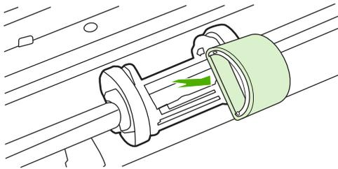
5. Position the new pickup roller in the slot. The circular and rectangular slots on each side prevents you from installing the roller incorrectly.
