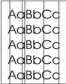
The photosensitive drum inside the print cartridge has probably been scratched. Install a new HP print cartridge. See [Replace the print cartridge on page 40](#).
