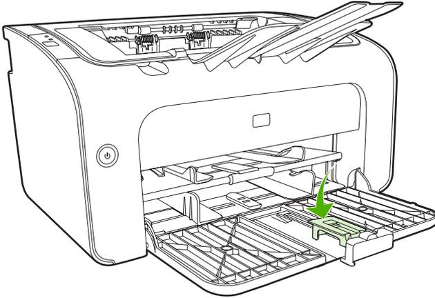
3. Insert the media into the device until it stops and then slide the adjustable media guide, with the tool attached to support the media.
