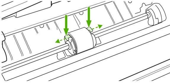
4. Gently pull the pickup roller up and out.
