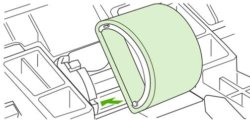
6. Rotate the top of the new pickup roller away from you until both sides snap into place.
