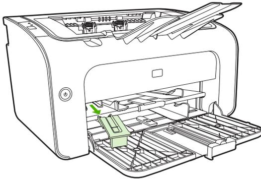
2. Attach the tool to the adjustable media guide.
