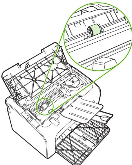
3. Release the small, white tabs on each side of the pickup roller, and rotate the pickup roller toward the front.
