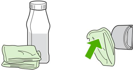
**⚠ WARNING!** Alcohol is flammable. Keep the alcohol and cloth away from an open flame. Before you close the device and plug in the power cord, allow the alcohol to dry completely.
