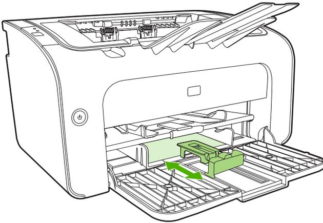
4. When finished printing with short media, remove the Short Media Extender tool and place it back in the storage slot.
