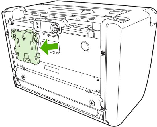
5. Insert the new separation pad, and screw it into place.
