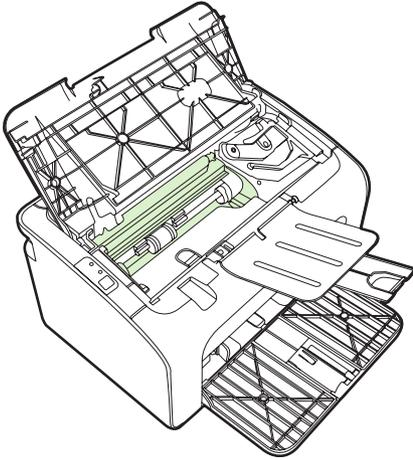
3. Replace the print cartridge, and close the print-cartridge door.
