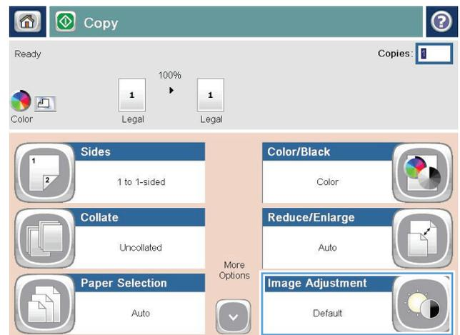
3. Adjust the sliders to set the **Darkness** level, the **Contrast** level, the **Sharpness** level, and the **Background Cleanup** level. Touch the **OK** button.
