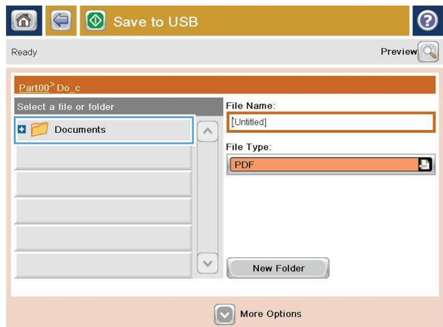
5. Enter the name for the file in the **File Name:** field. Touch the **OK** button. Select the file type from the **File Type** drop-down list. Touch the **OK** button.
