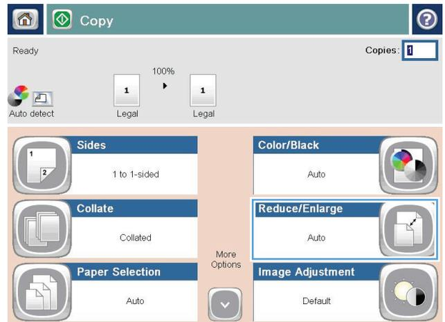
3. Select one of the predefined percentages, or touch the **Scaling** field and type a percentage between 25 and 200 when using the document feeder or between 25 and 400 when copying from the scanner glass. Touch the **OK** button. You can also select these options:
