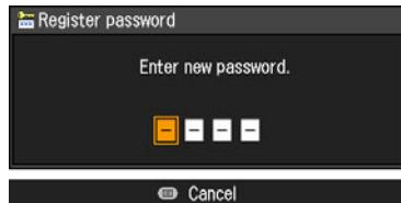
Enter a 4-digit password using [ $\wedge$ ] / [ $\lt$ ] / [ $\vee$ ] / [ $\gt$ ] (e.g.,  $\wedge\wedge\wedge\wedge$ ,  $\lt\lt\lt\lt$ ,  $\wedge\vee\lt\gt$ ). The 4-digit password is entered from the left to right digits, the password is automatically registered.
