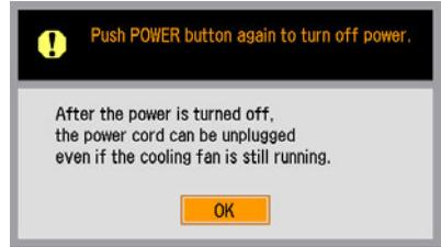
Press the **POWER** button again while the confirmation message is displayed. The lamp goes off, the [POWER] indicator starts flashing in red and the cooling fan starts.
