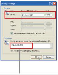
To designate proxy settings that will not use the proxy server when accessing the projector installed in the local area network, enter the IP address or domain name here.
