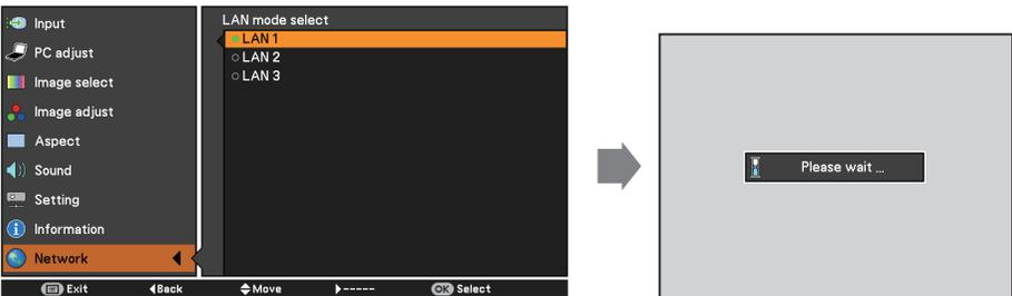
3. Select "Network setting" in the Network menu and press **OK** button, and then the LAN setting screen will appear and selected LAN settings will be displayed. Adjust each item to the setting environment. Consult your system administrator about the detailed settings.
