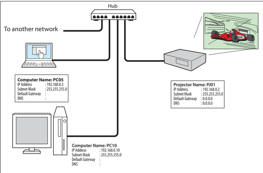
When the projector is connected to the computer directly without hub, the STP cross cable should be used.
