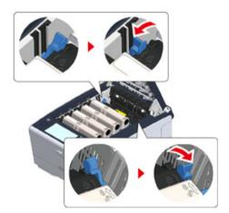
7 Hold the fuser unit handle and lift the fuser unit out of the machine.
