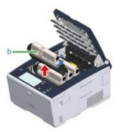
Hold the cartridge, pinch the tip of blue lever (c) of the toner cartridge, and turn it toward you until the tip aligns on the lug of the cartridge.
