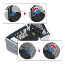
14 Replace the four image drums into the machine
