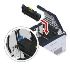
11 Tilt the lock levers on the both sides of the fuser unit.
