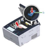
Tilt back the lock levers on the both sides of the fuser unit toward you.
