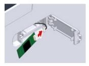
Install the wireless LAN module to the machine.
