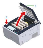
Remove the four image drums from the machine and place the image drums on a flat surface.
