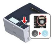
When the machine is turned on, the power switch LED lamp lights up.
