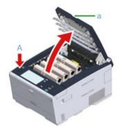
2 Remove the four image drums from the machine and place the image drums on a flat surface.
