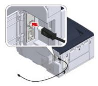
5 Pass the USB cable under the tab, and then close the interface cover.
