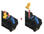
Hold the fuser unit handle and aligning the fuser unit to the grooves behind the toner cartridges, place the fuser unit into the machine.
