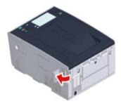
Insert one end of the USB cable into the USB interface connector on the machine.
