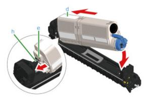
Hold the cartridge, pinch the tip of blue lever (g) of the toner cartridge, and turn forward until the tip aligns on the lug of the cartridge.
