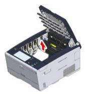
If paper jams in the fuser unit, press the jam release lever on the fuser unit and slowly pull the jammed paper toward you.
