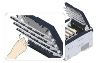
Do not use solvents, such as methyl alcohol or thinners. They damage the LED head.
