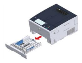
9 Slide the paper guide (a) to the width of paper to be loaded.
