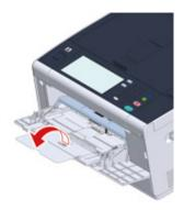
⚠ Adjust the manual feeding paper guide to the width of paper to be loaded.
