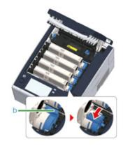
Lift the toner cartridge (c) from right side, and remove it from the machine.
