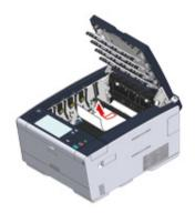
Hold the fuser unit (e) handle and place the fuser unit into the machine.
