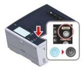
The "System moves to shutdown. Please confirm status when status LED is blinking." message is displayed on the touch panel, and the power switch LED lamp flashes at approximately one-second intervals.
