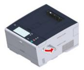
Spect the connector from the cover and connect with the wireless LAN module.
