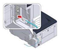
Pass the LAN cable under the tab, and then close the interface cover.
