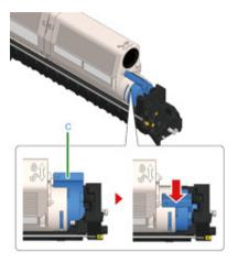
Lift the toner cartridge (d) from the right side, and remove it from the image drum.
