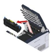
Tilt the lock levers on the both sides of the belt unit toward you and remove the belt unit by holding the lock levers.
