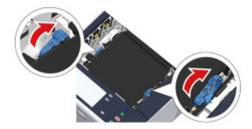
13 Hold the fuser unit handle and place the fuser unit into the machine.
