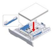
Secure the loaded paper with the paper guide.
