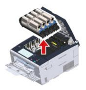
4 Cover the removed image drums with paper so that the image drums are not exposed to light.
