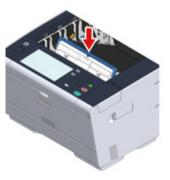
Turn the lock levers on the both sides of the belt unit forward.
