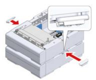
3 Slowly stack the machine on the additional tray unit aligning their back sides and right sides.
