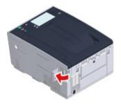
Insert one end of the LAN cable into the network interface connector.
