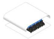
4 Pull out the jammed paper gently to the rear of the machine (the direction of the arrow) if an edge of jammed paper can be seen.
