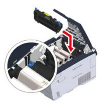
10 Push the levers on the fuser unit to lock.
