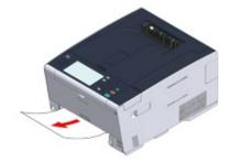
If jammed paper cannot be found, check the positions of paper guides and paper stopper in the tray and ensure that paper is correctly loaded.
