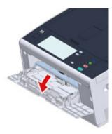
Pull out the paper support by holding the center part of it.
