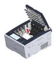
Hold the lock levers of belt unit and place the belt unit into the machine.
