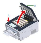
Remove the four image drums from the machine and place the image drums on a flat surface.
