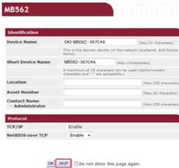
The screenshot shows the MB562 configuration interface. The 'Identification' section includes fields for Device Name (OK-MB562-367C4A), Short Device Name (MB562-367C4A), Location, Asset Number, and Contact Name - Administrator. The 'Protocol' section shows TCP/IP and NetBIOS over TCP both set to 'Enable'. At the bottom, there are buttons for 'OK', 'SKIP', and a checkbox for 'Do not show this page again.' The 'SKIP' button is highlighted with a red box.
