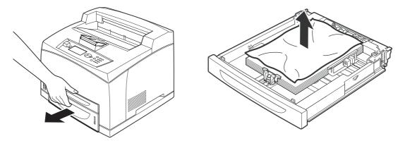
**2.** Examine the inside of the printer and remove any jammed paper.
