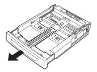
**5.** Squeeze the length guide and slide it to the desired paper size (1). Squeeze the right width guide and slide it to the desired paper size (2).
