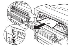
**3.** Raise the lever as shown in the diagram and open the cover B (1).
