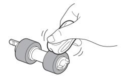
**4.** Turn the short tab (1) of the feed roller to the right and slowly push it onto the shaft of the paper tray.
