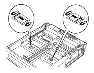
**4.** Hold the grip of the paper tray and pull its extendable part to the front until it reaches its maximum.
