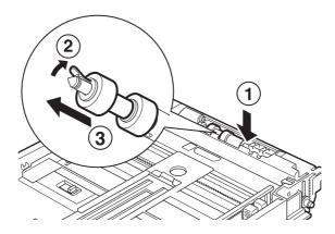
**3.** Wipe the rubber parts with a wet but well-wrung soft cloth.
